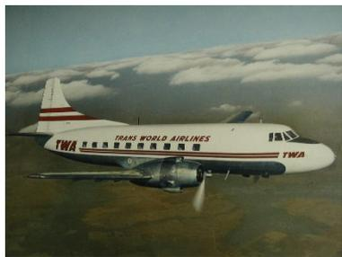
rear of the aircraft. The aircraft on the flight line that morning had tail number N-40416. It was powered by two Pratt & Whitney R-2800 CB16 18-cylinder radial engines each generating 2,400 horsepower. Normal cruising elevation was around 18,000 feet. Skyliner Binghamton had arrived in Albuquerque the night before after a flight originating in Fresno, California.
